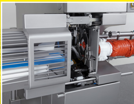
Shortest setup time due to comfort opening of front flap
