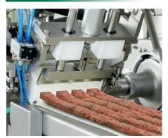
The automatic filling flow divider FST803 is an appliance for flexibly dividing fully identical filling flows in all production conditions. This guarantees accurate weight filling and hence an extremely consistent product quality. The filling flow divider is designed as an accessory to the vacuum filling machines and is directly fitted to the outlet of the machine.
