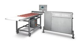
The shuttle conveyor SC260 is an addition to all single strand VEMAG production lines. The shuttle conveyor SC260 is used in all applications where products are portioned in a single strand and are transported in multiple strands. It can easily be integrated in VEMAG production lines. The shuttle conveyor performs up to 40 lifts per minute for a movement range of the retraction edge of 650 mm.
