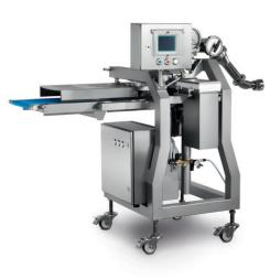
Discovering new ways - this was the force behind the innovative VEMAG Ball Control BC235. Fitted with opposed cutting plates, the Ball Control BC235 produces filled convenience products such as meat balls, croquettes, hamburger patties and many more in a fast and clean fashion. The selected form of the products per cycle has absolutely no influence on the accuracy of the portions - it is always exact right from the first to the last product. For a homogeneous appearance.
