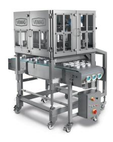
The current filling device for the simple portioning of viscous mixtures is exact, fast and reliable - whether for liverwurst, ground pork or creams. The cub edges remain clean, the filling quantities are identical for reproducible quality. The fully-automated line portions exactly to weight and on several lines into tubs, jars, bowls etc. The usual dripping is prevented using inner tube seals: Tub edges and conveyors remain clean, which reduces the rework significantly and perfects hygiene.
